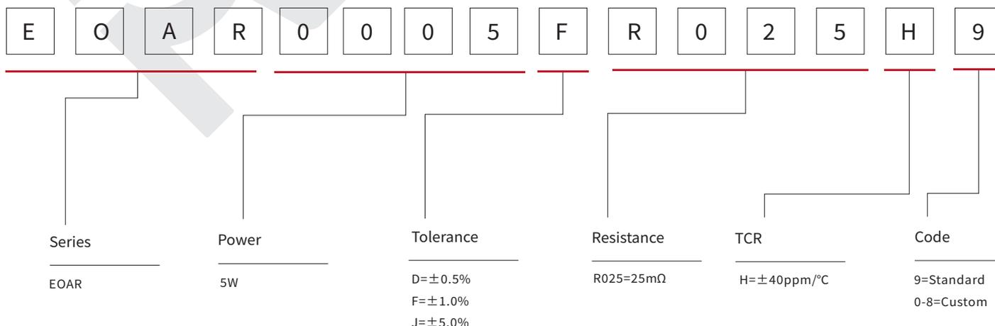
For higher/lower resistance, tighter tolerance, higher power, lower TCR and larger size, please contact us.
