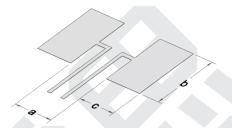
Not following the recommended solder pad design can seriously affect the temperature coefficient measurement results and current sensing accuracy!
